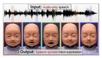
Fig. 1: **Dynamic animatronic robot facial expressions generated from speech.** The figure shows the system's capability to produce diverse and lifelike facial expressions in real-time, synchronized with the corresponding audio speech input. The waveform at the top represents the audio input, while the series of images below showcase the robot's facial responses at different time points.
